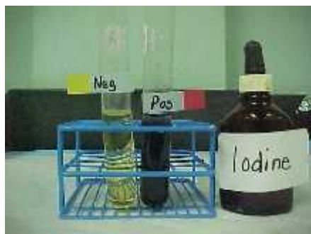
Fig 5.2: Test for starch
